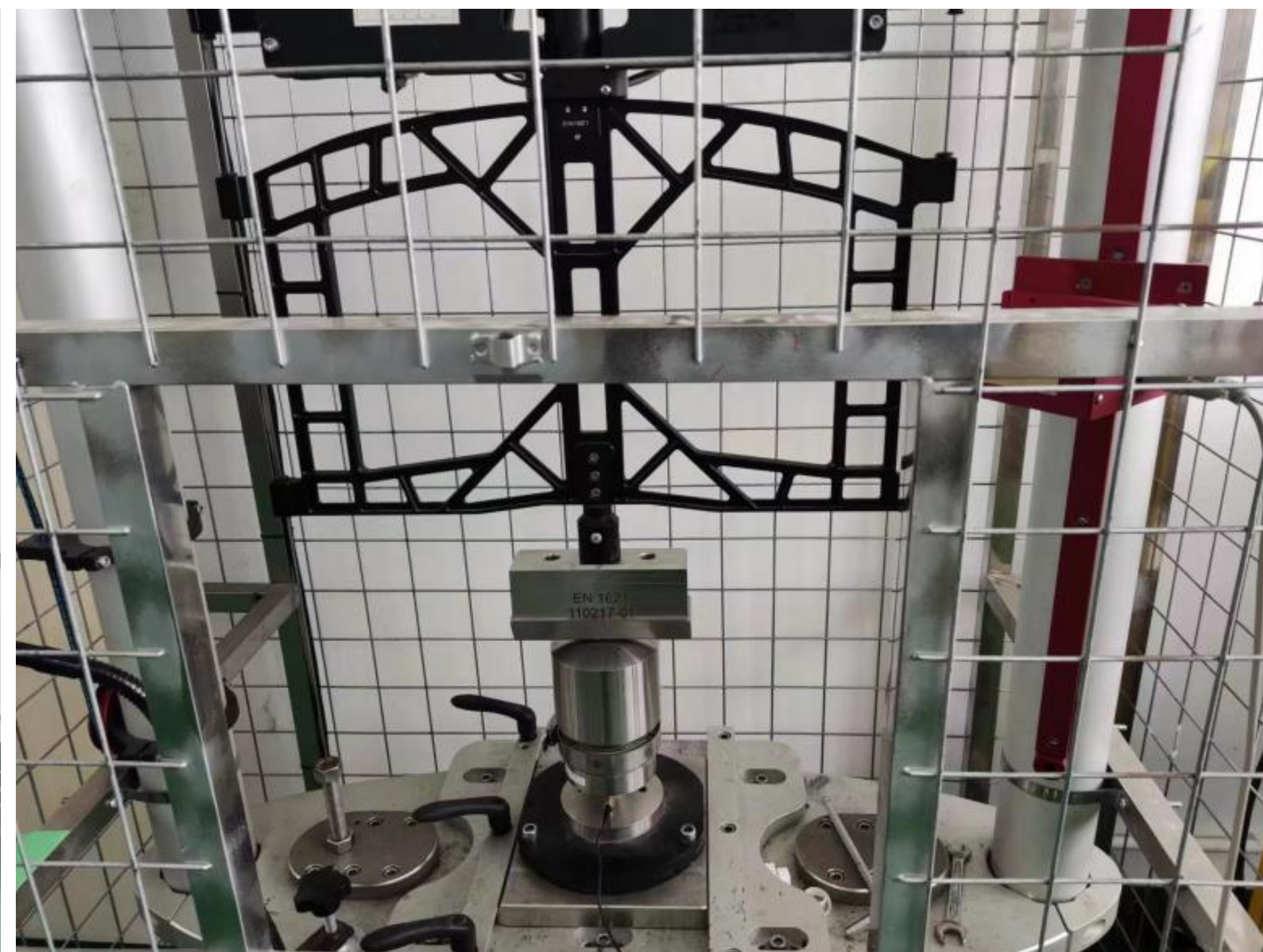
According to the testing standard EN 1621-1:2012 for impact tests of joint braces-Fall hammer and anvil
